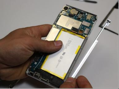
Remove the side bezels from each side, and remove the sim card cover.
