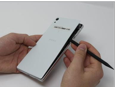
• Carefully remove the back panel of the phone with a plastic spudger, or other flat and thin wedge tool. Work your way around the perimeter of the case, loosening and prying gently, until there is sufficient distance between the panel and phone.
