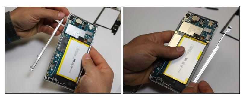
• Remove the side bezels from each side, and remove the sim card cover.
