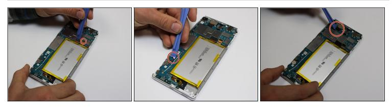
• Disconnect all four of the shown electrical connectors by gently prying up with the plastic opening tool.
