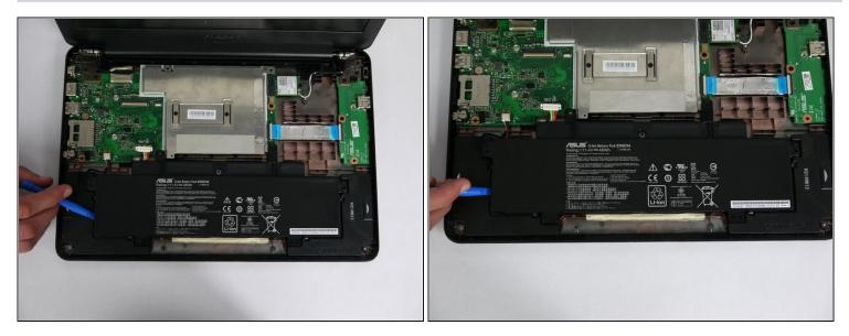
• At this point, using the plastic removal tool, lift the battery out of the shell.
