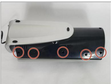
Start off by using a Philips #2 screwdriver to remove all 8 10mm exterior screws on the rear of the device.
