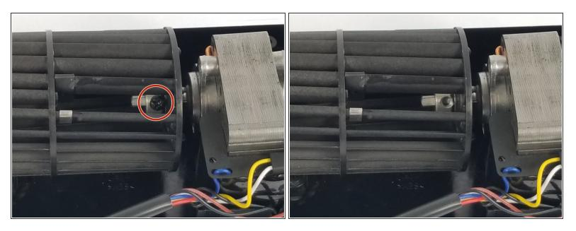
Loosen 5 mm screw at bottom of fan blade located inside the blades.
