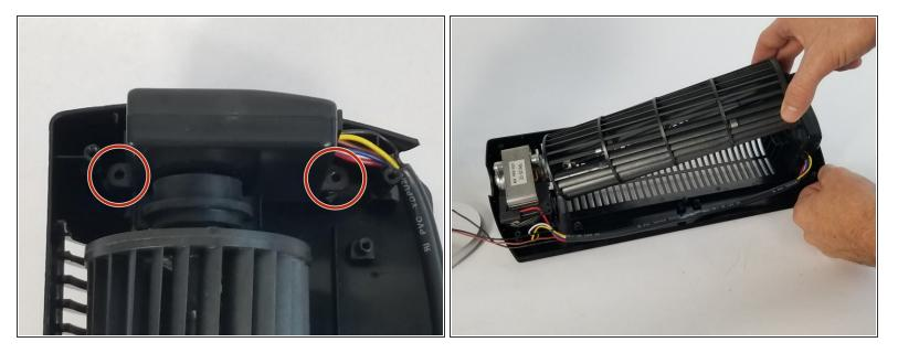
Remove fan blade after unscrewing top 2 screws located on each side of the covered board.
