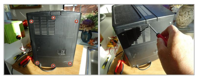
• The rear panel and side panels are attached with six phillips screws #2. Screw them out.
