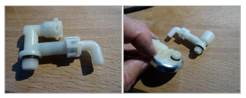
• The old safety valve - seen in the first photo already expanded - is screwed on the pump. It is replaced by a combination of safety valve and pressure balance valve. The diaphragm valve dampens the shocks of the pump, making the flow of water quieter and quieter.
