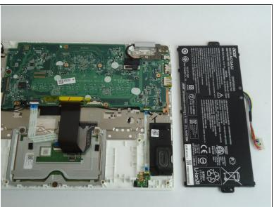
Carefully lift the battery from one side, and then lift it out of the laptop.
