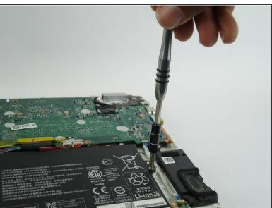
Unscrew the (2) two 3mm J0 Phillips head screws that hold the battery in place.
