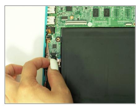
Detach the speaker cable from its fastener on the motherboard by pulling it out with your fingers or using a spudger.
