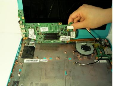
• Carefully lift the motherboard up towards the screen as if it was hinged on one side.
