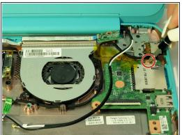
Remove the three 3mm screws from the surface of the motherboard using a Phillips Head 1.
