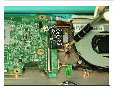
Remove the 3mm screw that holds down the Wifi mini-PCI card using a Phillips Head 1 driver.
