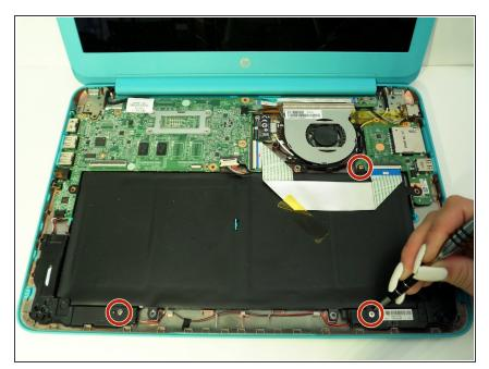
Remove the three 4mm screws around the perimeter of the battery pack with a Phillips Head 1 screwdriver.
