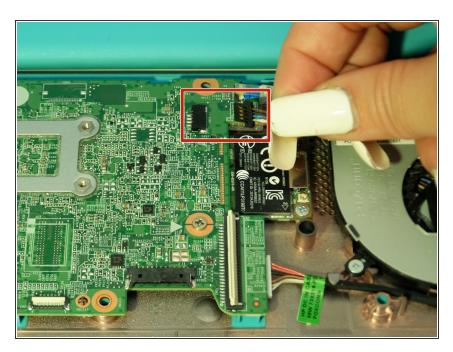
Using your fingers, pull the cooling fan cable from its fastener on the motherboard
