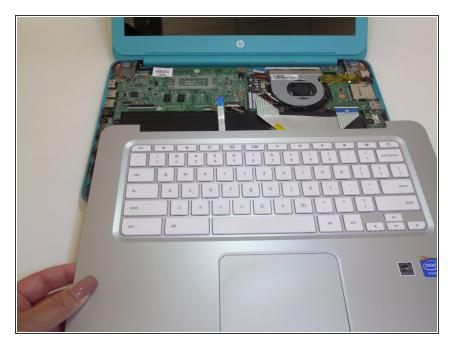
Lift the keyboard panel up and away from the CPU, completely revealing the mainframe.
