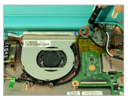
In the upper right hand corner of the device, remove the 6mm screw holding the PCB board in place by using a Phillips Head 1.
