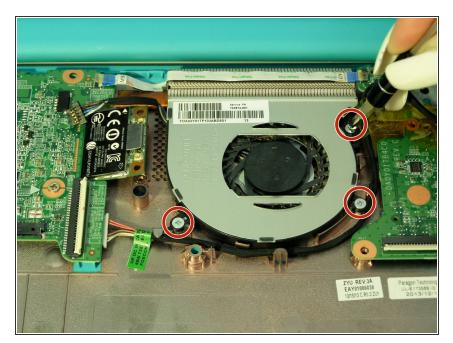
Remove the three 3mm screws that hold the cooling fan in place using a Phillips Head 1 driver.
