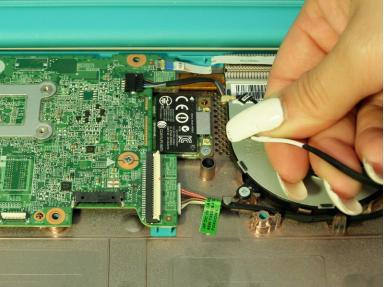
• Remove the two Wi-Fi antenna cables that are attached to the Wi-Fi card by pulling them up.
