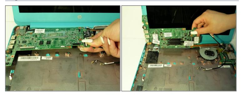
• Carefully lift the motherboard up towards the screen as if it was hinged on one side.
