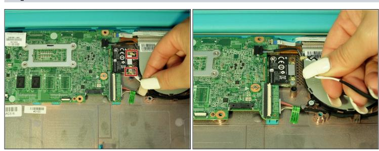
Remove the two Wi-Fi antenna cables that are attached to the Wi-Fi card by pulling them up.
