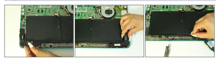
• Using your fingers, gently pry out the two L-shaped speaker panels from between the external casing and battery pack.
