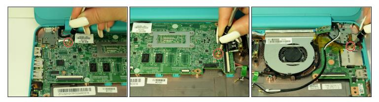
• Remove the three 3mm screws from the surface of the motherboard using a Phillips Head 1.
