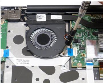
• Using the #1 Philips screwdriver, remove the two, 2mm screws securing the fan assembly.
