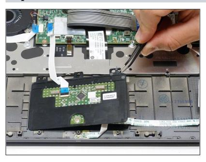
Now that the mouse pad is exposed, lift the assembly to remove the mouse pad.
