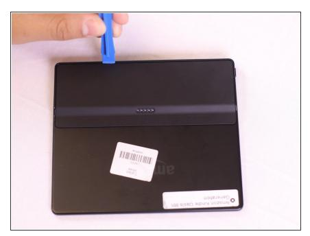
• Carefully wedge the plastic opening tool between the back panel and the device to free the clips holding the back panel and the device together.
