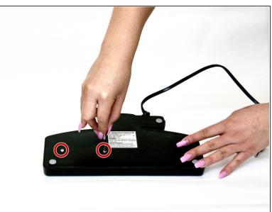
Using a PH #2 screw driver, remove the three 18mm screws on floor charger.
