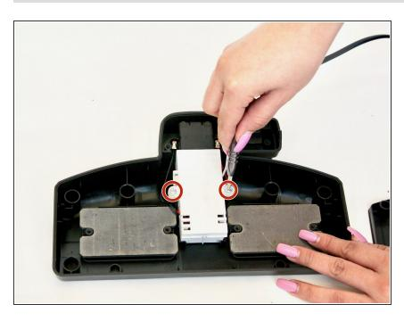
Unscrew the two 18mm screws on either side of the white battery cover with a PH #1 screw driver
