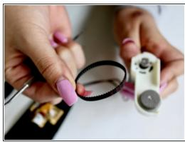
Use a metal spudger to lift the belt away from the mechanism.
