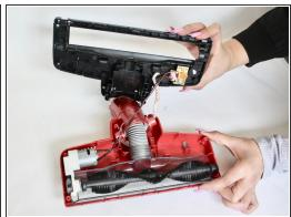
Using a firm grip, pull the two halves of the vacuum head away from each other until they are completely separated
