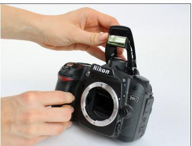
Using a plastic opening tool, pry open the cover.
