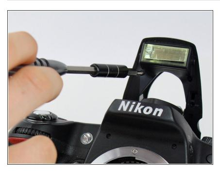
Use the #00 Phillips-head screwdriver to remove both 4.20 mm screws by rotating the screwdriver to the left.
