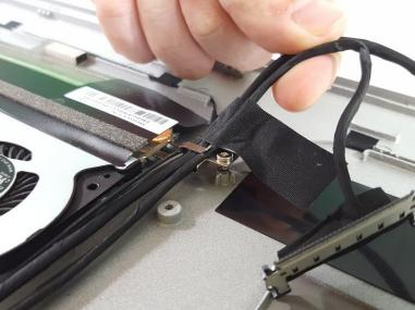
• With the Phillips screw driver using the number one head. Carefully unscrew the M2-6mm wire fastener, so the wires shown in the picture can be released from the rear casing.
