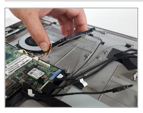
Lift the fans carefully out of the casing.
