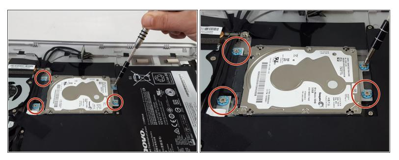
Using your Philips head screw driver with the number 1 head. Carefully unscrew the four M2-6mm screws that are circled in the picture.
