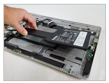
Carefully lift the battery from the rear casing.
