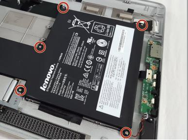
• Using the Philips screw driver with the number 1 head. Carefully unscrew the six M2- 6mm screws that are circled in the picture.
