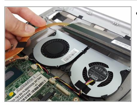
With the screws detached carefully lift the heat sink off the CPU on the motherboard.
