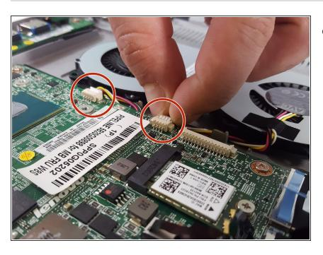
Carefully remove the power plugs connecting the fans to the motherboard.
