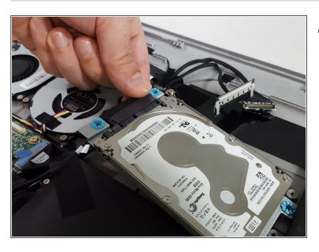
Now carefully lift the hard-drive that is still attached to the boot from the rear casing.
