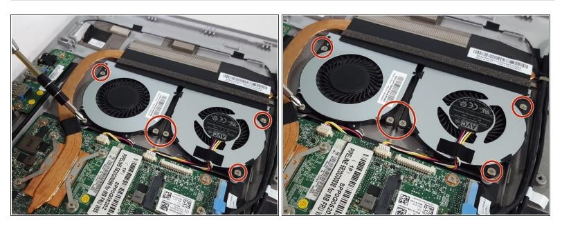
With a Phillips #1 screwdriver, unscrew the six M2 6mm screws located around the fans, as shown.
