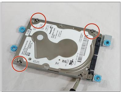
Now that the hard-drive is detached from the rear casing you will still have to detach the hard-drive from its boot. Again using the Philips screwdriver with the number one head. Carefully unscrew the four M2-6mm screws that are circled in the picture.
