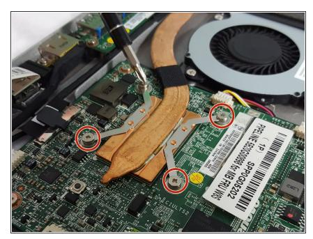
With the Phillips screwdriver using the number one head carefully unscrew the four M2 6mm screws circled in the picture.
