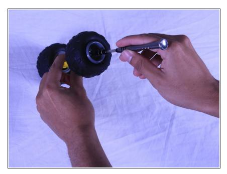
Place the new wheel onto the car and screw into the center of the wheel.
