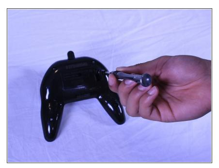
• Take the Philips screwdriver and twist the screw counterclockwise on the middle right side.
