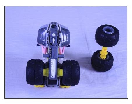
Place the new wheel into the car and attach the new screw
