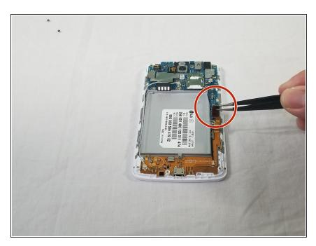
Using the precision tweezers set lift the copper tab located on the right side of the device.
