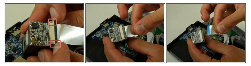
Disconnect the ZIF connector, by using your fingernail to lift up on the small locking flap. Then pull the ribbon up and away, out of the connector.
