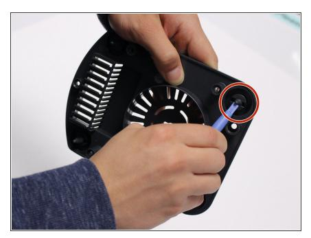
Push the stopper on the suction cup foot through the bottom panel using the iFixit plastic opening tool.
