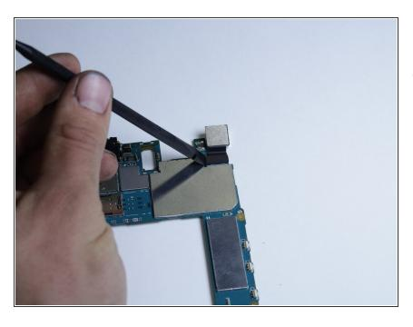
Using a plastic spudger, disconnect the camera from the motherboard. To reassemble your device, follow these instructions in reverse order.
