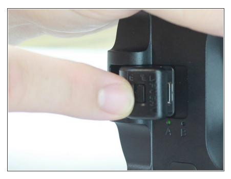
Slide the latch to the right to unlock the current connector.
