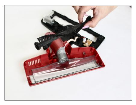
Remove brush from inside the vacuum head.
