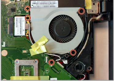
Using the Phillips #0 Screwdriver, remove the nine 2mm screws at the marked locations.
