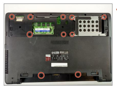
Using the Phillips #0 Screwdriver, remove the ten 2mm screws at the marked locations.
