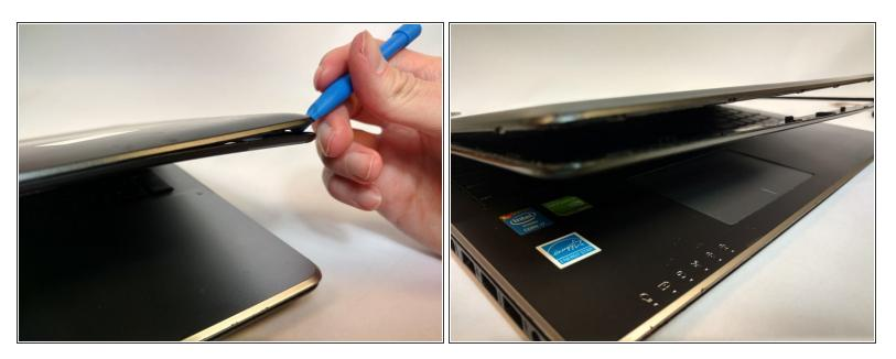
• Using the plastic opening tool, open the front cover of the laptop.
