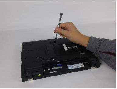
• Loosen (do not remove) the 14.0mm screw in the DIMM slot cover with a Phillips #2 screwdriver.
