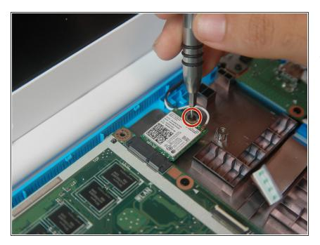
• Using the Phillips #000 screwdriver, unscrew the 4mm screw.
