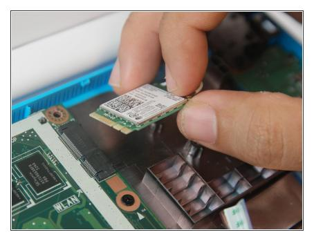
Gently remove the wireless card making sure to not damage the connecting port.
