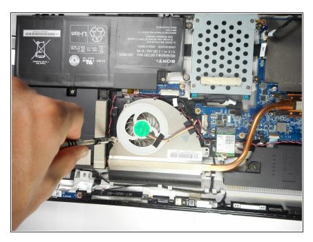
Remove two 6mm screws located on both sides of the fan component using a Phillips #1 screwdriver.
