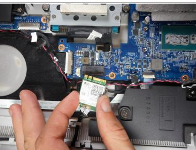
Gently detach the wireless receiver and place it somewhere it does not obstruct the speaker assembly.
