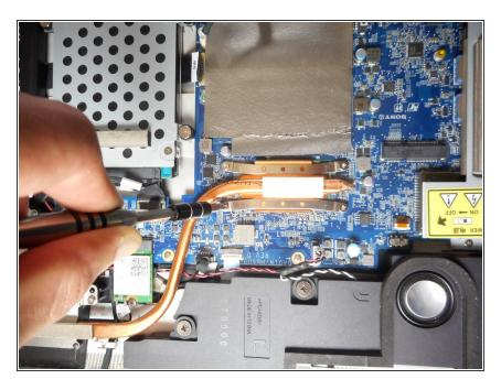
Remove four 9mm screws from the fan attachment located on the motherboard with a Phillips #1 screwdriver.
