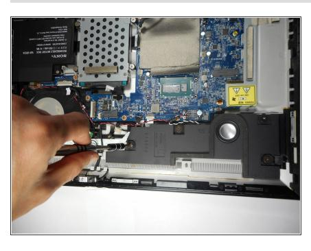
Remove a total of four 8mm screws with the Phillips #2 screwdriver from the speaker located below the motherboard.
