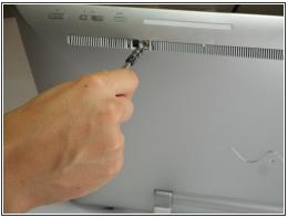
Remove the two 5mm screws on the back of the device using a JIS 0 screwdriver.
