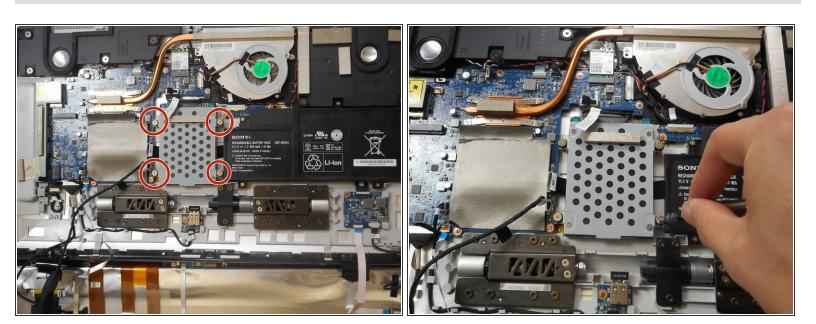
• Locate the 13mm screws for the hard drive and use the JIS 0 screwdriver to unscrew.
