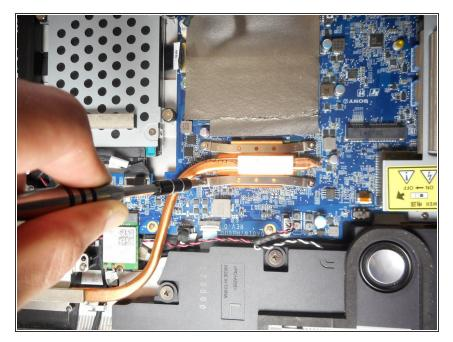
Remove four 9mm screws from the fan attachment located on the motherboard with a Phillips #1 screwdriver.
