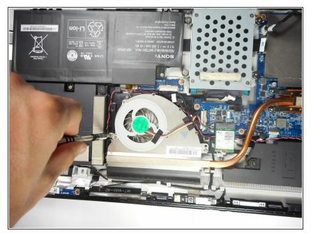
Remove two 6mm screws located on both sides of the fan component using a Phillips #1 screwdriver.
