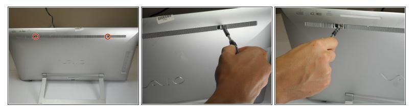
• Remove the two 5mm screws on the back of the device using a JIS 0 screwdriver.
