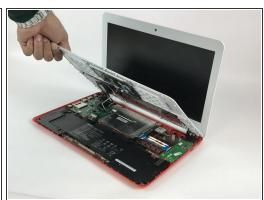
Gently wedge the spudger in between the bottom of the device and the keyboard, and carefully pry
