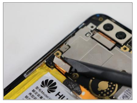
Using a spudger, gently pry up the connector near the left edge of the motherboard.
