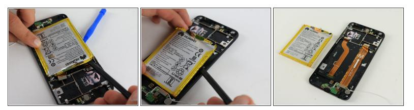
• Once all the adhesive has been removed from the battery, use the spudger and plastic opening tools to gently pry the battery away from the frame.
