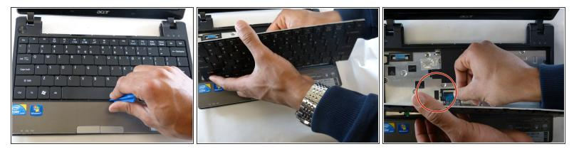
• Remove the keyboard with a plastic opening tool or spudger.
