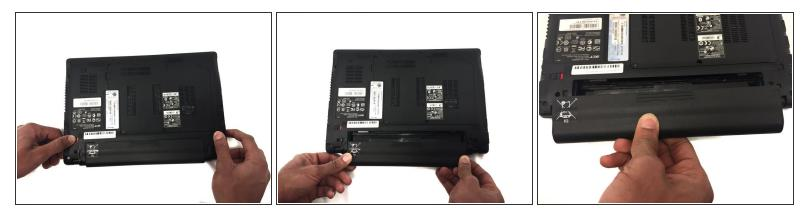
• Hold the battery release button, and pull the battery out of the laptop.
