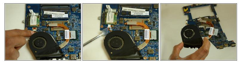
Carefully remove the fan from the motherboard by detaching the plastic insert as seen in the pictures
