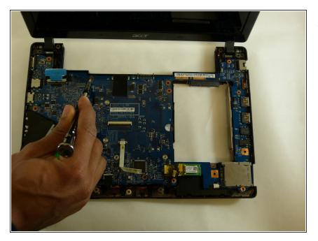
After removing the motherboard, turn it over so that the back side is facing you.
