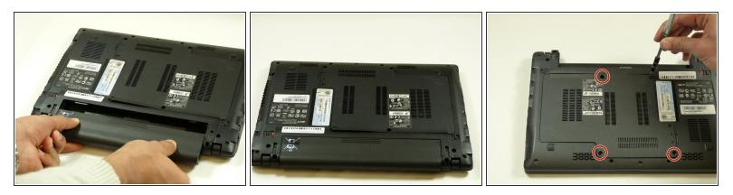
Remove the device's battery before beginning.
