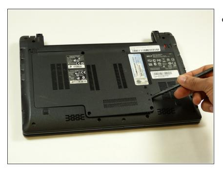
Pry open hard drive cover using the Spudger tool.
