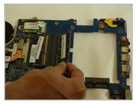
After RAM memory card is released from the motherboard, hold the RAM card on a 45 degree angle and remove the card.
