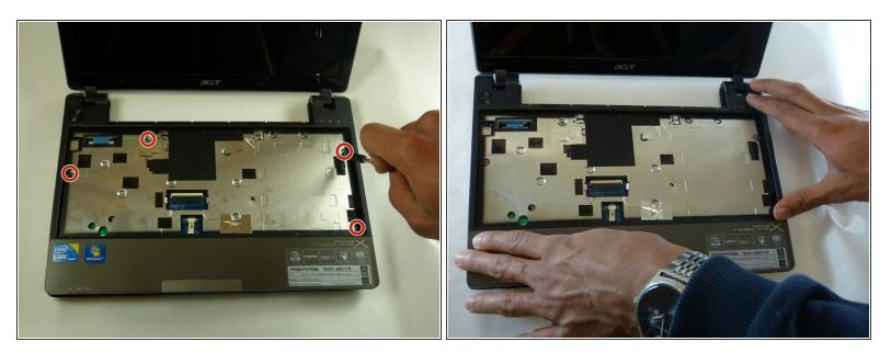
• Use a Phillips #0 screwdriver to remove the 4 screws from the motherboard shield.
