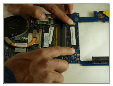
• To release the RAM from the motherboard, press both of the metal prongs on the sides of the RAM.
