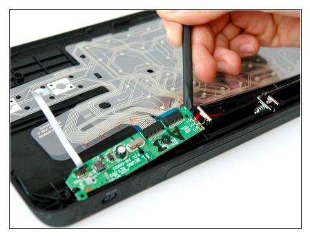
• Lift the green card up using the flat end of the plastic spudger.
