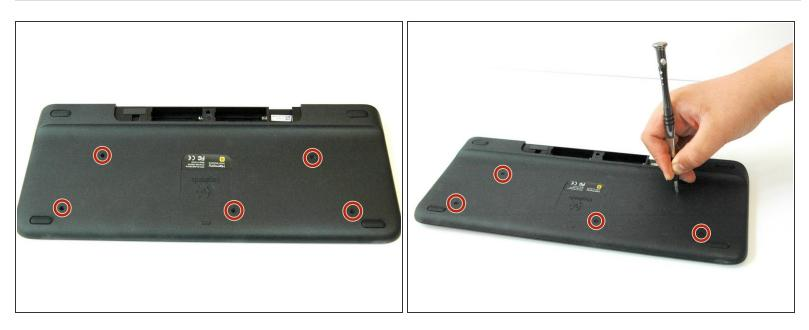
Unscrew all five 4.0 mm screws, using Phillips #1 screwdriver.
