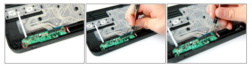
• Unscrew the two 4.0 mm screws on either side of the green card using a Phillips #1 screwdriver.
