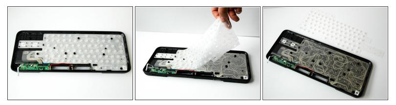
• Lift and remove the white rubber sheet that lays over the keyboard pet flexible PCB.
