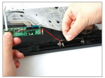
• Grip and lift the battery wire bar out of the battery compartment, using your thumb and index finger.
