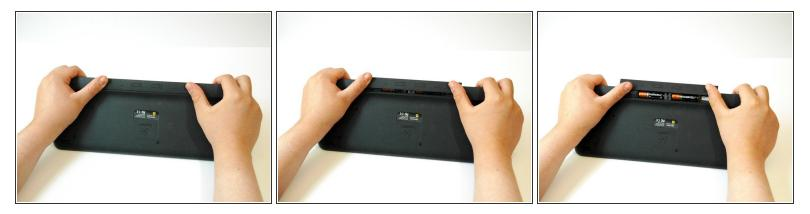
• Press and slide up on the upper battery latch, using both thumbs.
