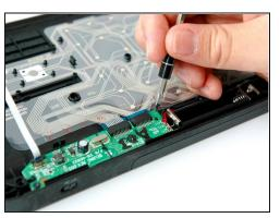
• Unscrew the two 4.0 mm screws on either side of the green card using a Phillips #1 screwdriver.
