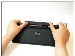
• Press and slide up on the upper battery latch, using both thumbs.
