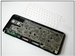
• Lift and remove the white rubber sheet that lays over the keyboard pet flexible PCB.
