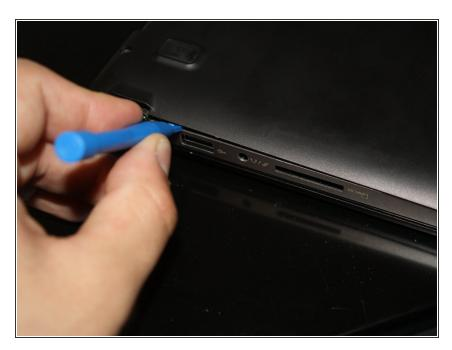
Use a plastic opening tool to open the components of the laptop. In order to do this, insert the plastic opening tool in between the two covers then pry open.
