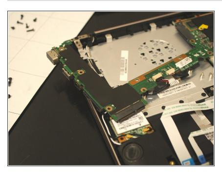
Desolder the headphone jack or completely replace the secondary motherboard chip.
