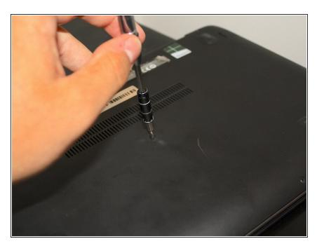
Remove the 9 1.2mm phillips head screws on the bottom of the computer using the smaller Phillips head screw driver.
