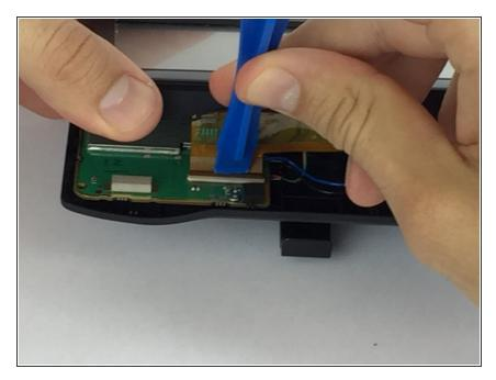
• Carefully use the spudger to flip open the ZIF connector.
