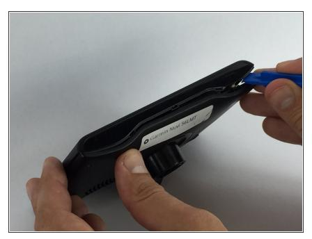
• Find the crevice where the front and back of the device meet.
