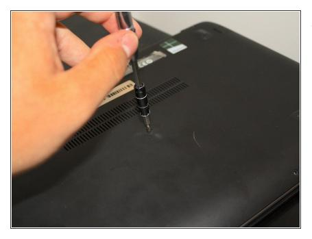
Remove the 9 1.2mm phillips head screws on the bottom of the computer using a small Phillips head screw driver.
