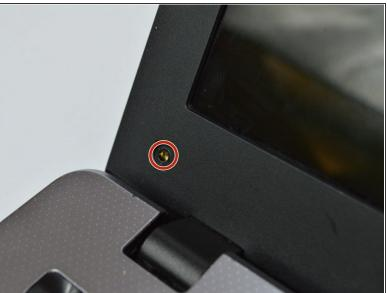
Remove the two 5mm screws at each bottom corner of the display using a Phillips #0 screwdriver.
