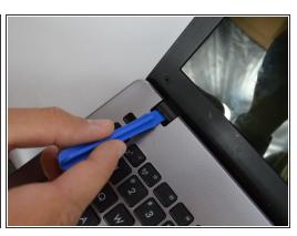
After the two screws are removed, use a plastic opening tool to remove the black cover around the screen.
