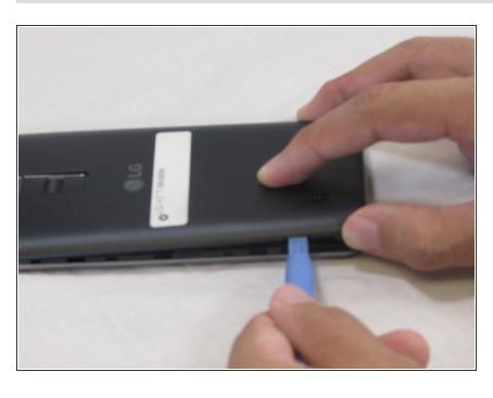
Insert a plastic opening tool into the notch and lift the back cover upward while holding the bottom portion of the phone down to remove it.
