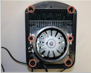
Using the Phillips #1 screwdriver, remove the 6 screws (13 mm long, 6 mm wide).
