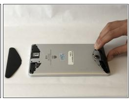
Use either your finger or a metal spudger to lift both the top and bottom black covers on the back of the tablet.
