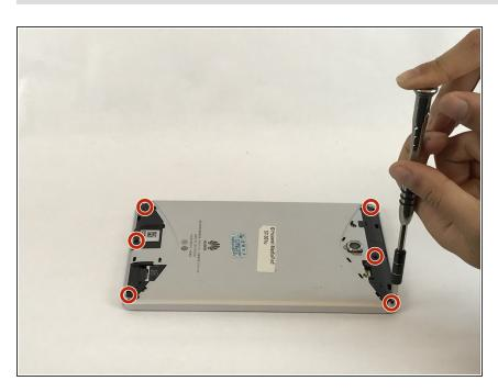
Use a Phillips (J000) bit screwdriver to remove the 6 (2 mm) screws located at the top and bottom of the tablet.
