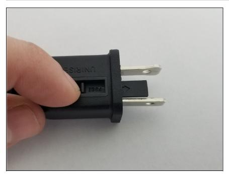
Open fuse cover by sliding access cover on top of attachment plug.
