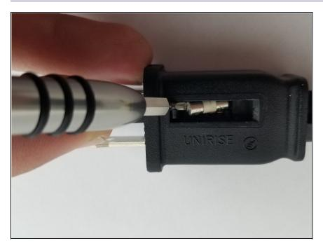
Install replacement fuse by first placing the end of the fuse into the fuse receptacle which is opposite of the blades of the plug, then carefully push in the other end. (Only push against the metal end of the fuse, not the glass center portion)
